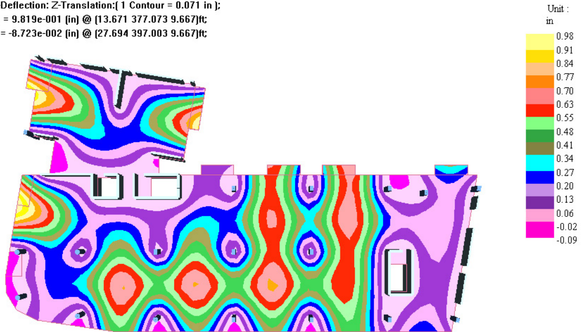
FIGURE EX4-1 DEFLECTION CONTOUR OF SLAB WITH CRACKING
